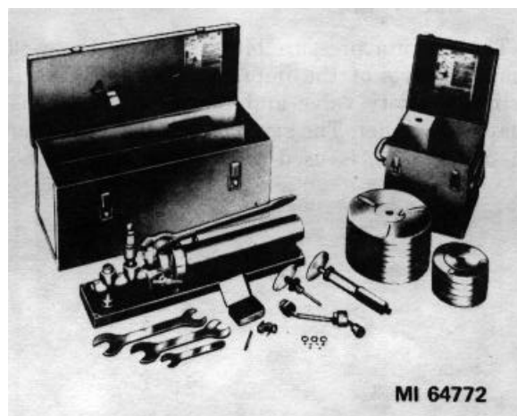
Figure 1-13. Portable dual-range deadweight tester assembly.
