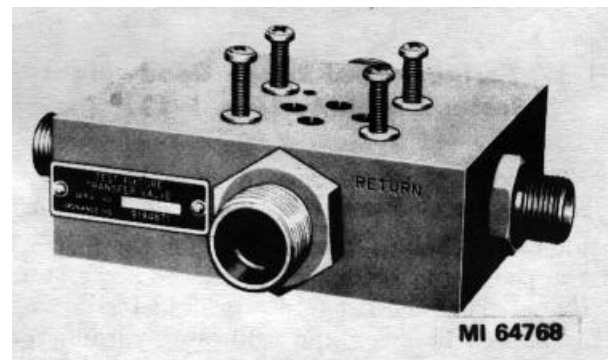
Figure 1-9. Transfer valve test fixture.
